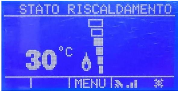
If the water temperature is lower than the one set on the display, the burner ignition sequence will start:
